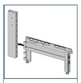
a) Insert base leg into lowest level of upright. Ensure rear lugs are pointing upwards.
