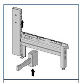
b) Use Rubber Mallet to tap base leg firmly upwards into upright. Ensure base leg is tightly fitted into base leg.
